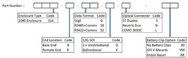
Note:- The End Location Code dictates the orientation of the 12G-SDI signal flow. So "R" denotes Transmitter and "B" denotes Receiver. In the event of an "X" (Transceiver) option, the Remote and Base units are handed.
