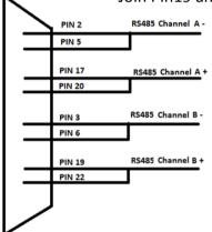
For RS485 with termination systems, follow the diagram below (typically used for long distance transmitting or single RS485 transceiver systems)
