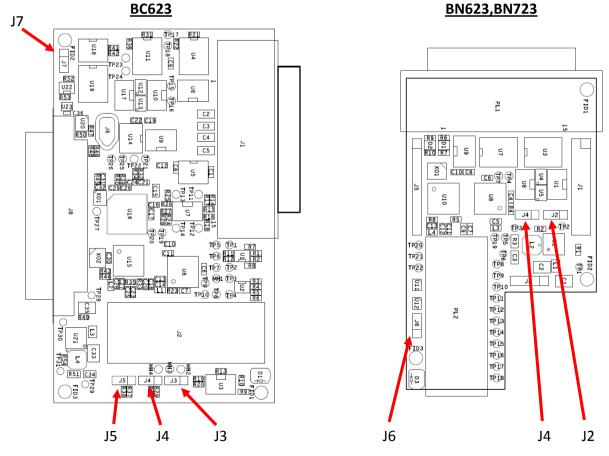
Note: Pin 1 is shown here as a square end on the connector. The cards have additional annotations for these links.
