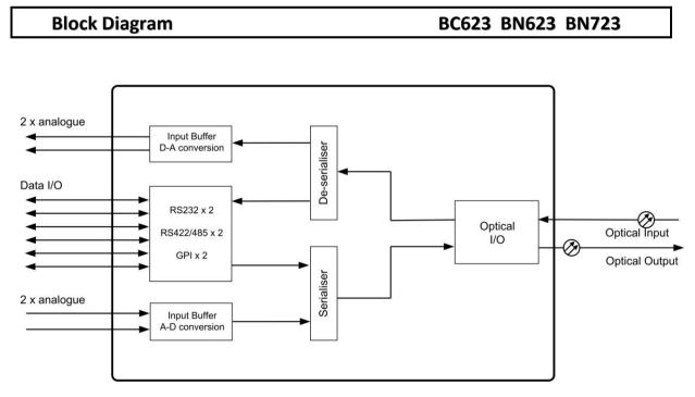
Note: the BN723 doesn't have the analogue audio inputs or outputs.
