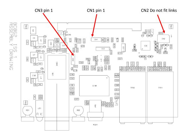
Note: Pin 1 is identified by a chamfered corner on the connector's white rectangle and by a square solder pad on the other side of the card.
