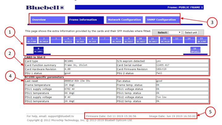
The Frame page displays more detailed information about the BC100i frame itself, and about all the cards inserted in the frame. The tabular page layout is consistent for all card types, though some fields will be empty depending on what data the cards can provide.
