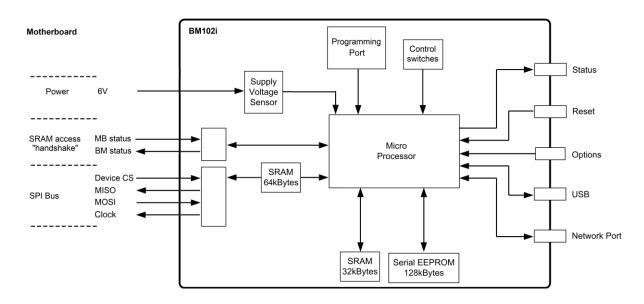
The frame's motherboard (BC100i or BC160i) has a microprocessor which gathers all data from all the cards and SFPs inserted in the frame. All of this data is passed down to a 64KB SRAM on the BM102i via SPI protocol. The BM102i's microprocessor then reads the data from the SRAM and transmits it for network monitoring over the network port.
