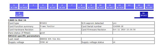
Example 2: Confirms the network card's data in slot 16. Serial number, PCB issue and firmware version - This information may be needed when contacting Bluebell with any technical issues that arising with the card. Last reset displayed on the network card is independent to that show on the frame page (slot 0).
