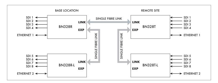
The example shows a pair of BN328s at each end of the single fibre link. At the remote site, the BN328T-L encodes four SDI signals and Ethernet data onto Low Band wavelengths, which are then passed by a fibre patch into the BN328T. As this optical signal uses different wavelengths to the BN328T, it can be multiplexed with the High Band wavelengths of the BN328T, enabling eight SDI signals and two separate Ethernet streams to the encoded onto the single fibre link.
