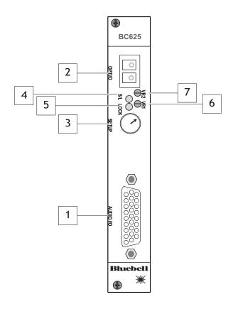
1. **AUDIO I/O** – all audio connections are made via the hi-density 26-pin female Dsub connector. All audio inputs and outputs are electronically balanced and at line level, nominally 0 dBu  $(0.775 \, V_{rms})$ .
