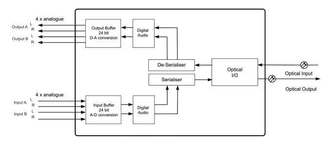
The four analogue inputs are electronically balanced, and will accept a maximum level of +24 dBu (ref. 1 mW into 600 ohms). A-D conversion is 24-bit, 48 kHz sampling rate. Post-conversion, the four audio inputs are converted into two AES3 signals before modulation onto the optical carrier.
