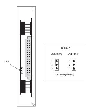
The jumper position sets the digital output level relative to an analogue signal level of 0 dBu.
