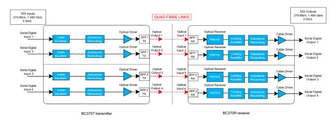
In this application, a BC370T will typically be installed at a remote camera location and a BC370R at the base location. Four independent SDI signals applied at the inputs of BC370T will be transported over separate optical links, and can be recovered at the SDI outputs of the BC370R. The video signal in each channel may be of any of the supported SDI standards.
