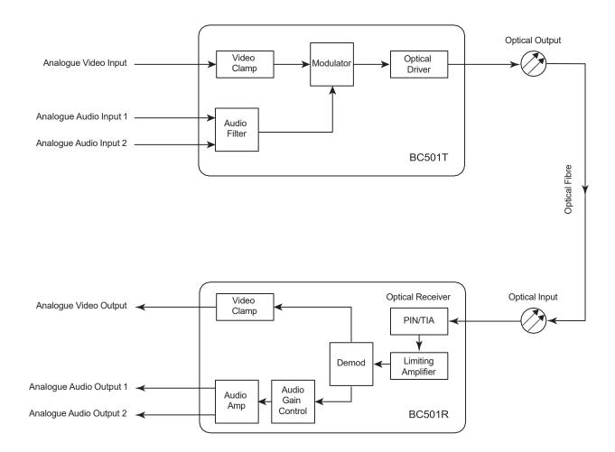
A BC501 system uses a single-wavelength optical signal over fibre to provide a robust long-distance interconnection between two widely-separated locations. The interconnection carries a multiplex of composite video and two channels of analogue audio.
