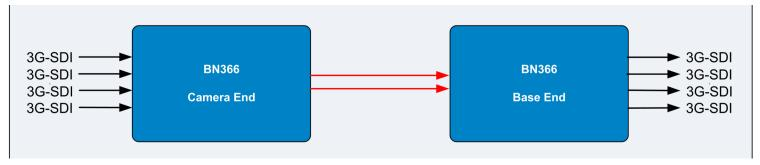
The BN366 carries four independent 3G-SDI signals over two fibres to give transparent high performance 4K links. Each BN366 multiplexes two separate wavelengths or services onto each fibre. Each wavelength is independent. In the case above four signals are being transmitted in one direction over two fibres.
